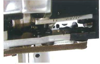
確定磨刀托架 P7-17 在上方定點 Confirm the knife holder, P7-17, is right on the above fixed point.
