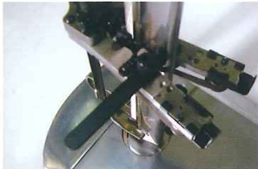
調整磨刀托架 adjustment whets the knife bracket
