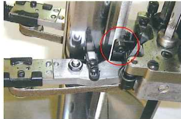
左蹄鐵上方螺絲調整 Left hoof iron above the screw adjustment
